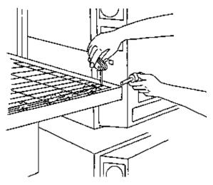
4. Remove conveyor drive chain cover as shown.
